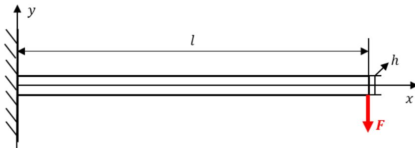
The MEMS beam is composed of a  $\text{SiO}_2$  layer and a Cr track on top. The cross section of the MEMS beam is shown in the figure below.
